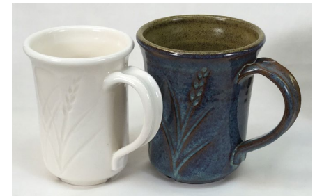
Left: Polar ice at cone 6 with a clear fritted glaze. Right: M390 stoneware at cone 6 with Alberta Slip glazes.
